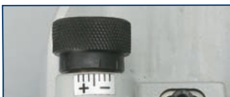
1 Tracer point with micrometric adjustment.
